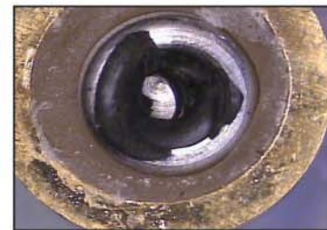
After 50,000 test cycles, the traditional O-Ring shows obvious signs of wear damage.
