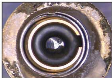
The SATURNO™ O-Ring attachment remains in excellent condition after 50,000 test cycles.
